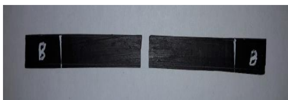
Fig -4: Bending Test Specimen after fracture
