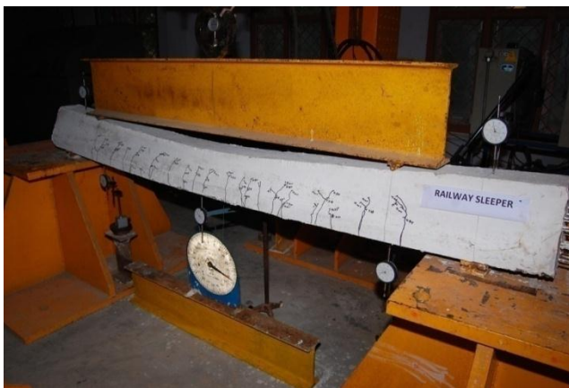
Fig.8. Crack Pattern of GPC Sleeper
