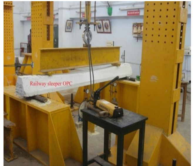
Fig.6. Experimental Setup of the Sleeper (OPC)
