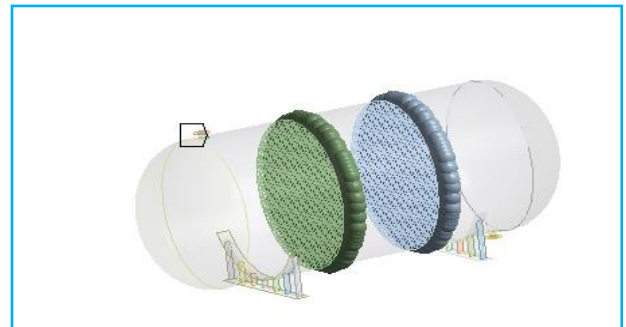
Figure-17: showing all point masses on all tube-sheets
