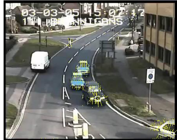
Figure 6: Key point of object using SURF or key descriptor
