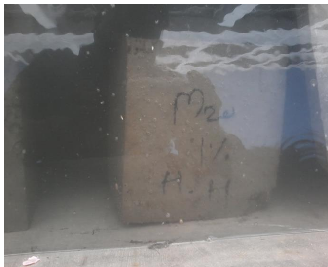
Photograph: 5 Curing Of Concrete Block
