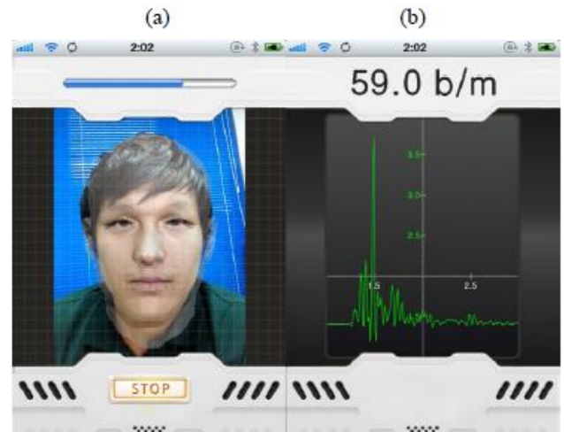
Figure . The screenshots of FaceBEAT. (a) FaceBEAT supports overlaid guide view on the recording. (b) FaceBEAT shows the estimated heart rate and the FFT results to user
