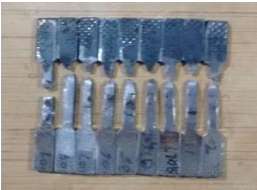
Fig-2:- Specimens After Tensile Test.
