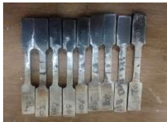
Fig-1:- Specimens Before Tensile Test.
