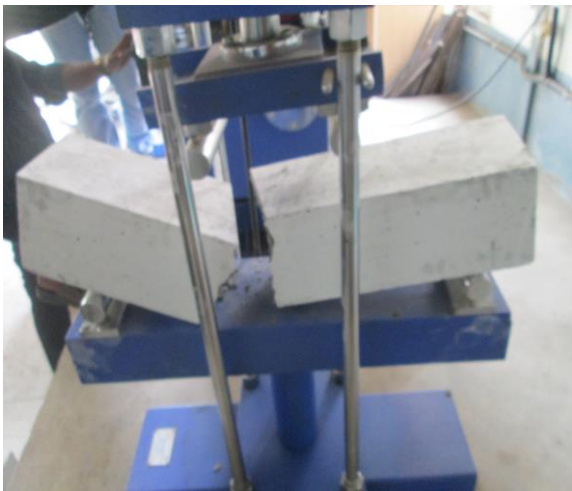
Fig -5: prism specimen tested for flexural strength
