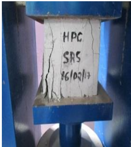
Fig -3: cube specimen tested for compression strength
