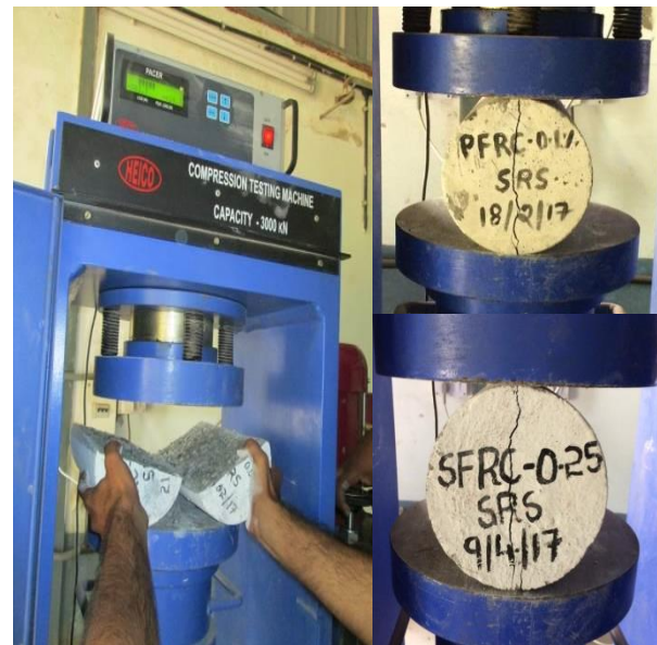
Fig -4: cylinder specimen tested for split tensile strength
