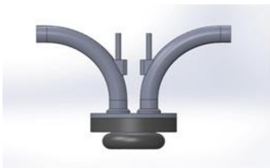
Fig 1. Front view of assembly of valves, piston, intake manifold and combustion chamber.
