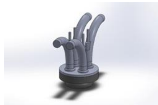
Fig 4. Isometric view of assembly of valves, piston, intake manifold and combustion chamber.
