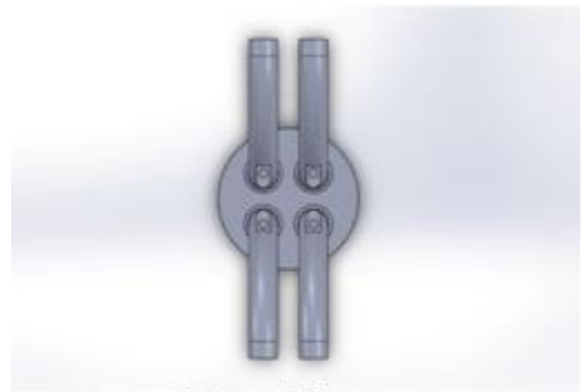
Fig 2. Top view of assembly of valves, piston, intake manifold and combustion chamber.
