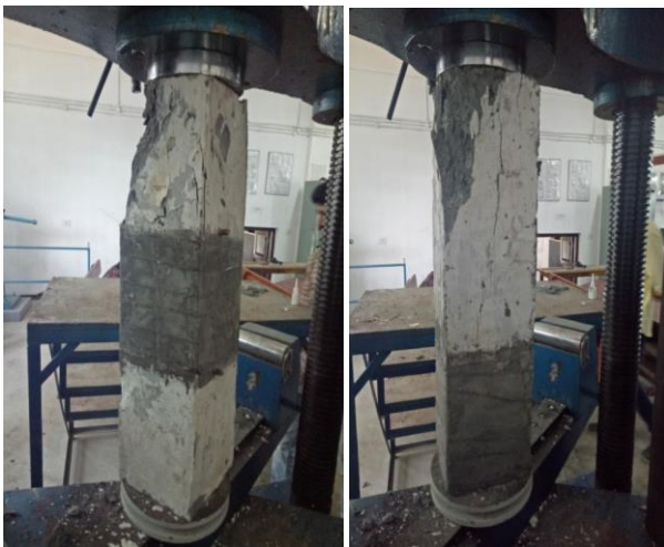
Columns wrapped with SSWM
