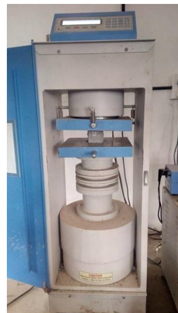
Fig - 2: Testing of mortar cubes in compression testing machine.
