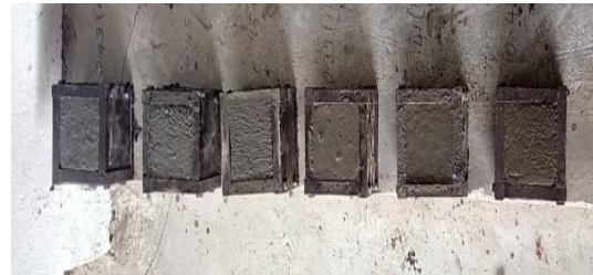
Fig - 1: Casting of cube specimens.
