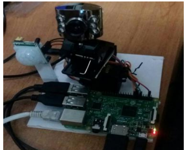
Fig -2: Raspberry Pi Installation Setup
