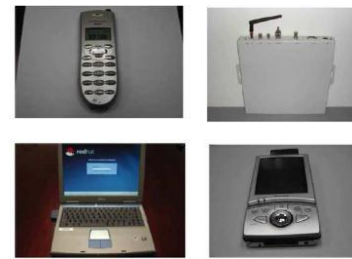
Figure 3.2: Examples of mesh clients: (a) Wi- Fi IP Phone, (b) Wi-Fi RFID Reader, (c) Laptop (d) PDA.
