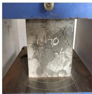
Fig -2: Compression test for cubes of M70 grade concrete in compression testing machine.
