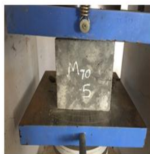
Fig -2: Compression test for cubes of M70 grade concrete in compression testing machine.
