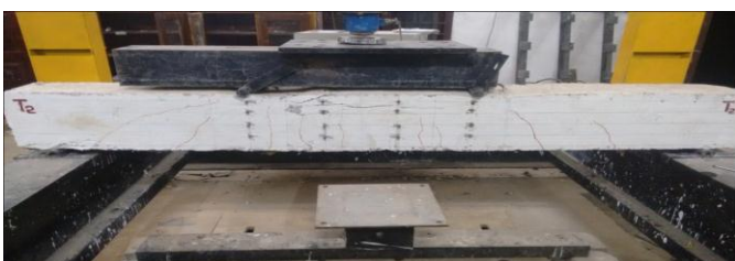
Fig-8 Crack pattern for beam having middle layer of thickness 100mm (T1)
