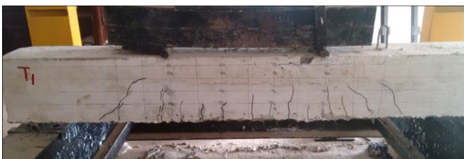
Fig-8 Crack pattern for beam having middle layer of thickness 100mm (T1)
