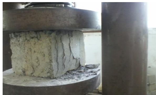
Figure-2 Testing of concrete cube specimen
