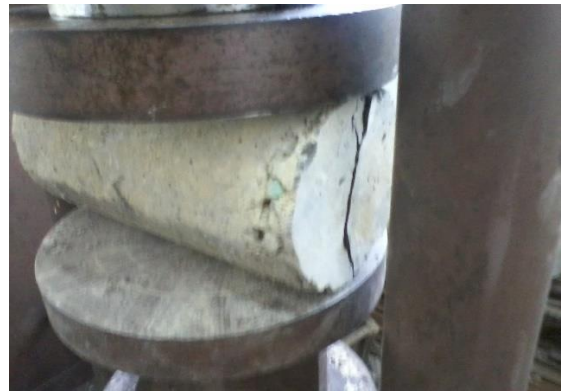
Figure-3 Testing of concrete cylinder specimen
