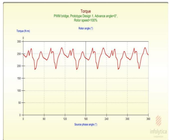
Fig -14: torque profile with standard stamping
