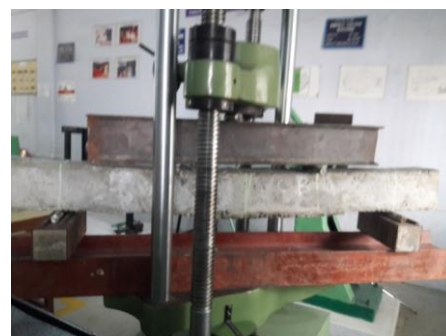
Fig- 3: Flexural strength test on RCC beam specimen
