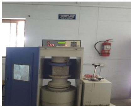
Fig- 1: Compression strength testing machine
