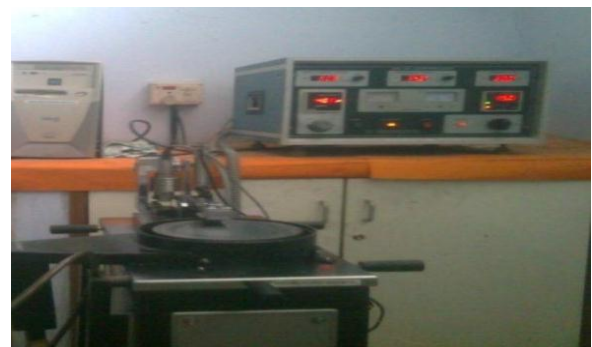
Fig. 1 Experimental Setup of Pin-on-disc Tribometer
