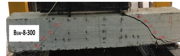
Fig -9: Crack pattern of BSW-8-300
