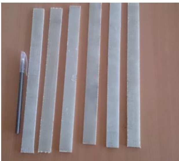
Fig -5: Prepared specimen for tensile test
