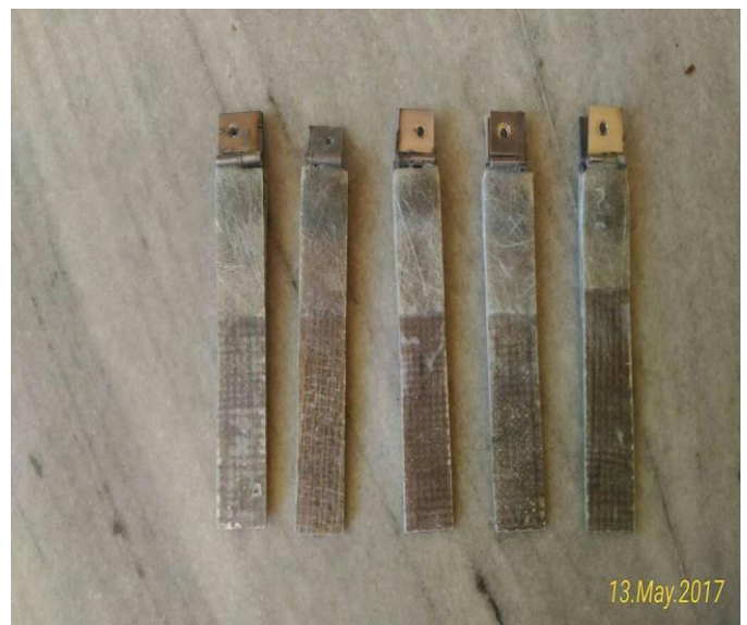
Fig -6: Specimen for mode I fracture toughness test
