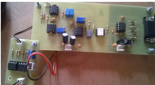
Fig 3: ECG sensor circuit
