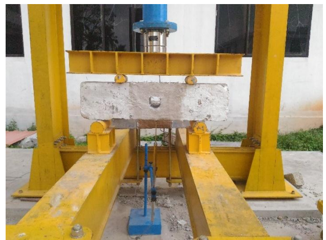
Fig Beam with GFRP wrapped inside the hole and on the surface
