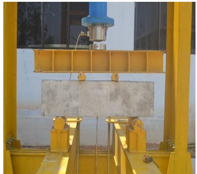
Fig Control beam without opening (CB1)
