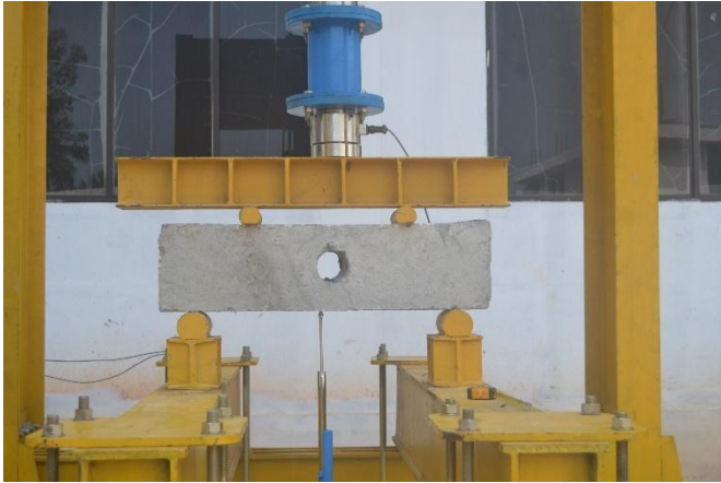
Fig Control beam with opening (CB2)
