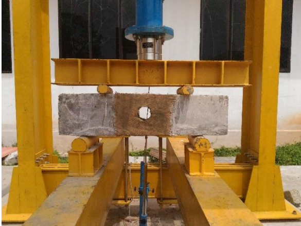
Fig Beam with AFRP wrapped inside the hole and on the surface
