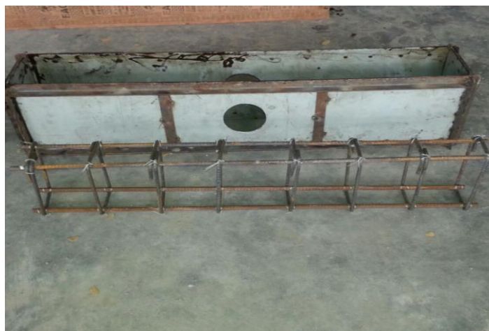
Fig.2.1 Reinforcement cage of the beam along with the specimen mould
