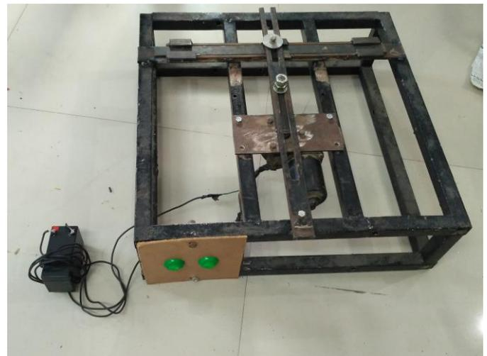
Chart -1: Crank and slotted lever mechanism
