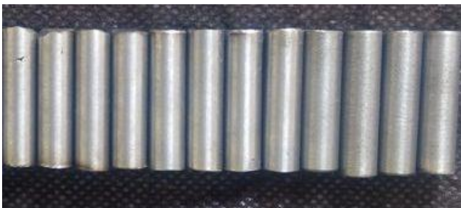
Fig 4: Cylindrical pins (30mm x 8mm) prepared for pin on disc test
