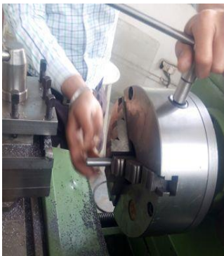
Figure 2. Preparation of test pins
