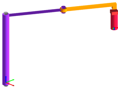
Fig-12: 3D Model of 4-Axis Adept-1 SCARA Robot
