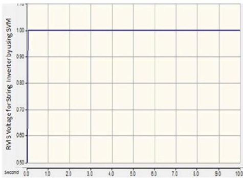
Fig-16: RMS-output of string inverter using SVM.
