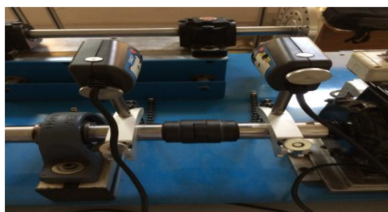
Fig.2 Structure of the laser alignment system with dual PSDs
