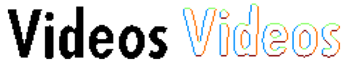
Fig.4 .eHOG representation. Sample text (left) and four types of edge points represented in four different colors (right). Note that the number of edge points in blue is roughly equal to that in orange, and so for green and crimson.
