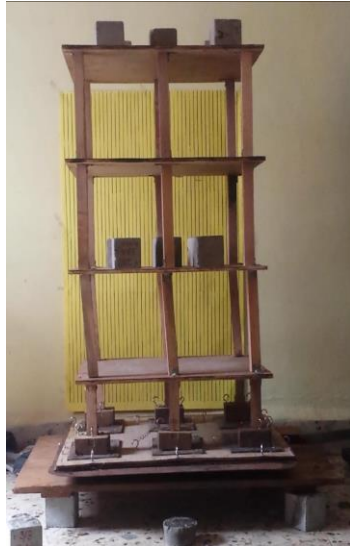
Fig -7 Deflections on left side when building is provided with springs acting as dampers & 2nd & 4th floor (Arrangements)
