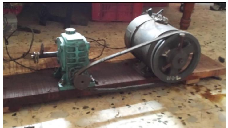
Fig -6 Modified motor & gearbox arrangement
