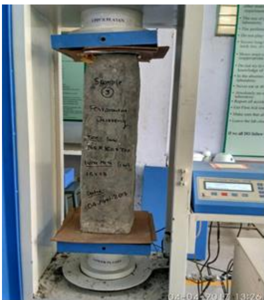
Figure 5 Axial loading Test Setup
