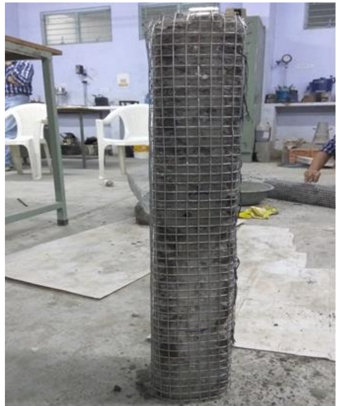
Fig - 3 Wrapping of wire mesh
