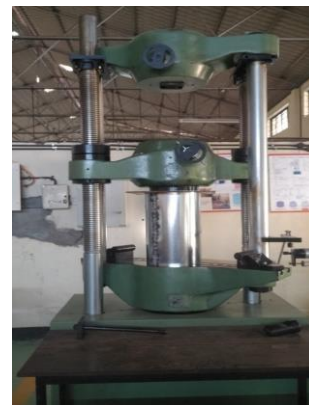
Fig -1: Experimental setup for buckling test
