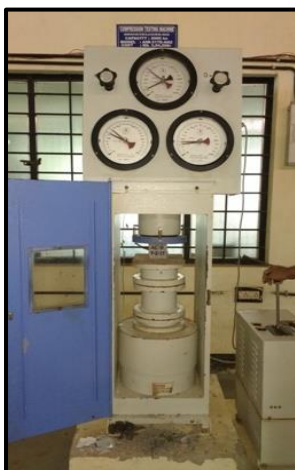
Fig -5: Test set-up Fig -6: Mortar Cubes under loading
