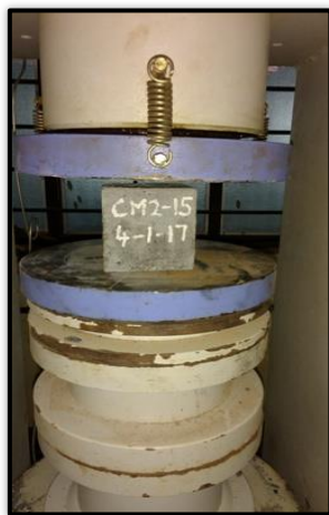
Fig -5: Test set-up Fig -6: Mortar Cubes under loading
