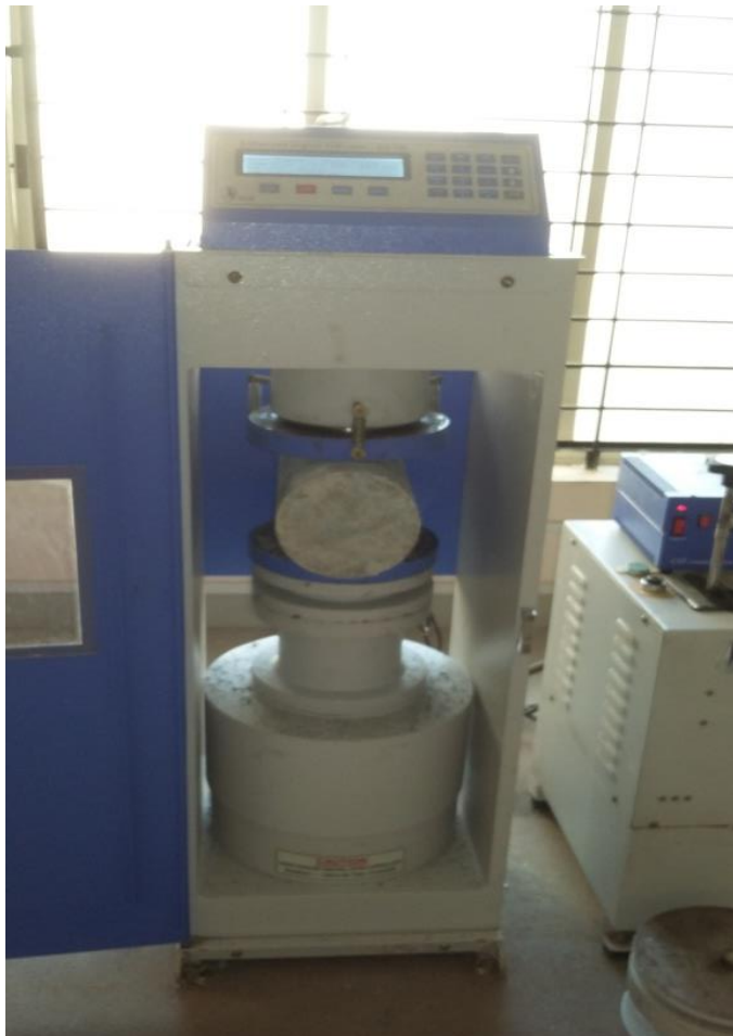
Fig 2: Testing of cylindrical specimen for tensile strength
