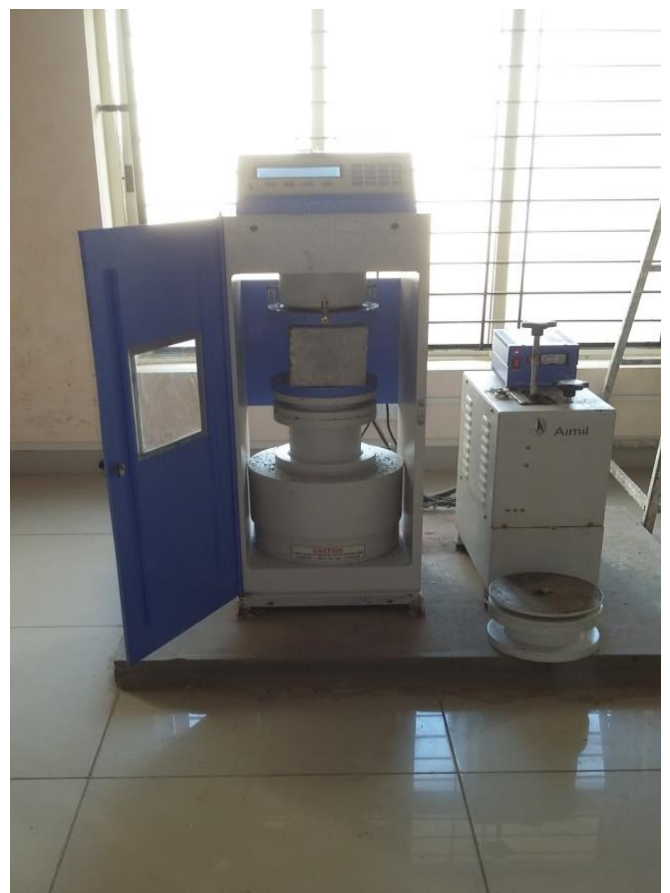
Fig 1: Testing of cube specimen for compressive strength
