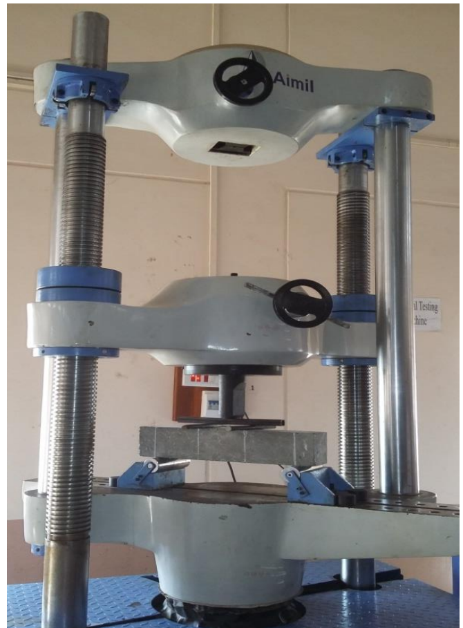
Fig3: Testing of beam for flexural strength
