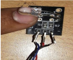
Fig.2: Illustration of Pulse Oximeter sensor
