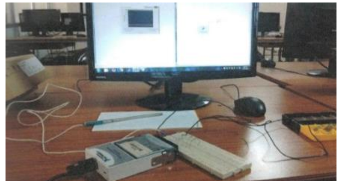
Figure -2: Experimental setup of J- type thermocouple connected to DAQ through a resistor to obtain faulty temperature readings.
