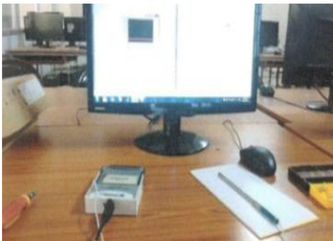
Figure -1: Experimental setup of J- type thermocouple connected to DAQ to obtain normal temperature readings
