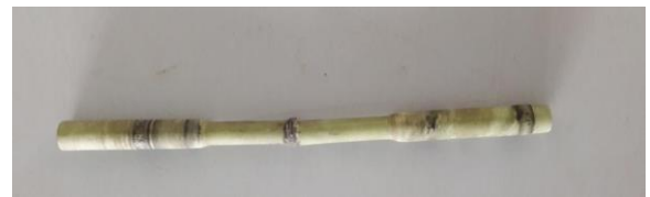
Fig: 4 - Unshotpeened specimen after fatigue
