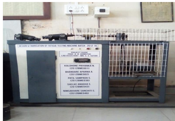
Fig -3: Fatigue testing machine
