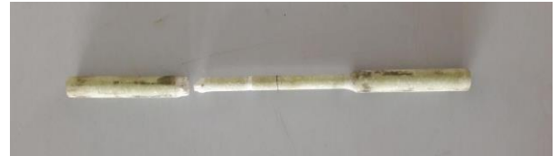
Fig: 5- 6 min shot peened specimen after fatigue
