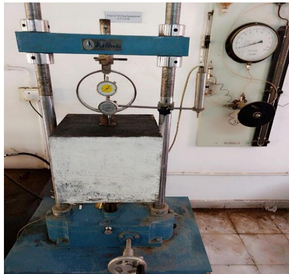
Fig -4: Model tank mounted on triaxial machine
