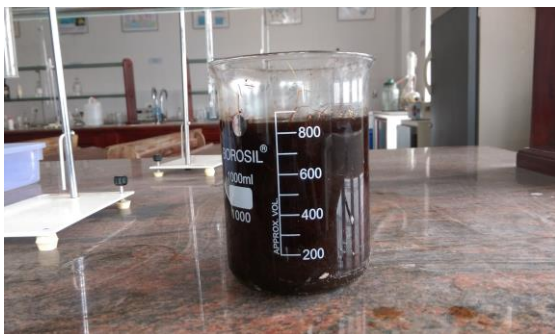
Fig.3. Coir fibre dipped in Sodium hydroxide solution
