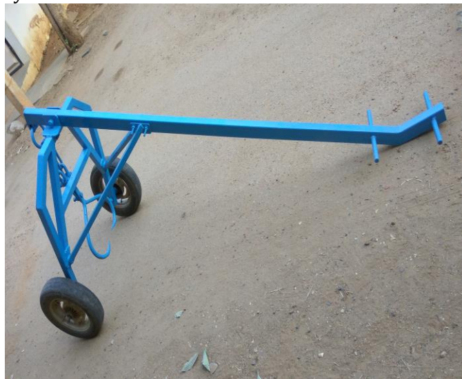
Fig. 13 Fabricated Log pulling arch
