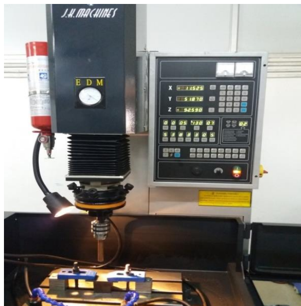
Fig -2: ZNC25 Die Sinker EDM machine setup with tool
