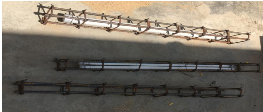
Figure 1: Reinforcement Cage for Beam Specimens
