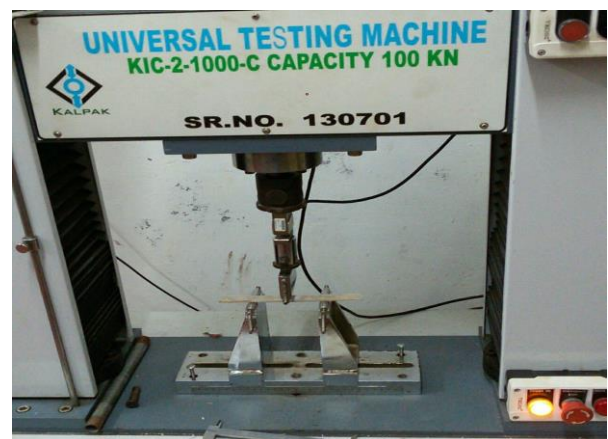
Fig -3: Bending Load Test
