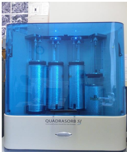
Fig -1: Quantachrome Apparatus for performing BET Analysis
