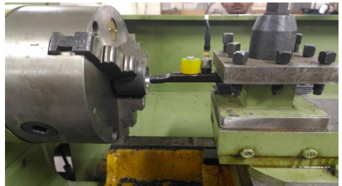
Fig -1: Damper setup on boring tool
