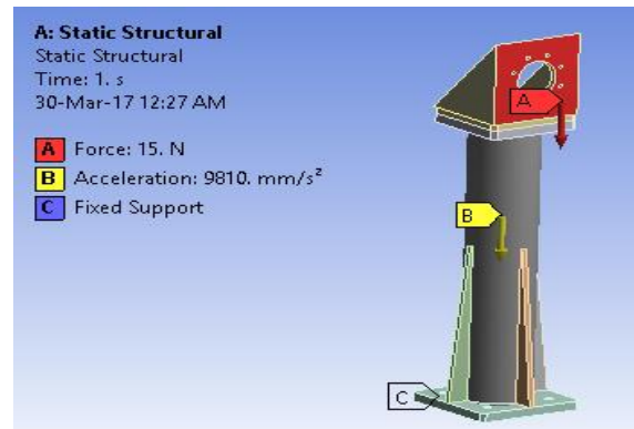
Fig-3: Loading Condition of mounting bracket.
