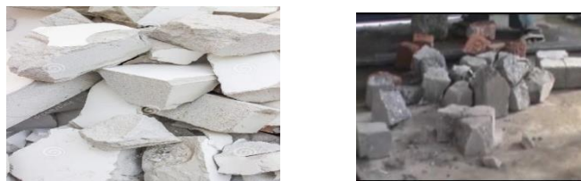
Fig. 5.1: Fly ash brick broken brick structure
