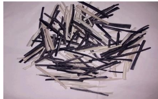
Figure- 4: E-Waste fiber
