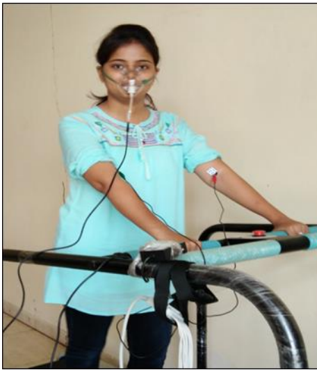
Fig-2: Acquisition of Reference respiration signal using thermistor
