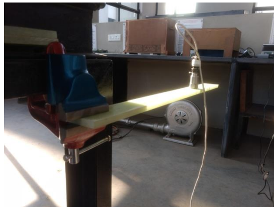
Fig-2 Experimental setup for crack detection in cantilever beam
