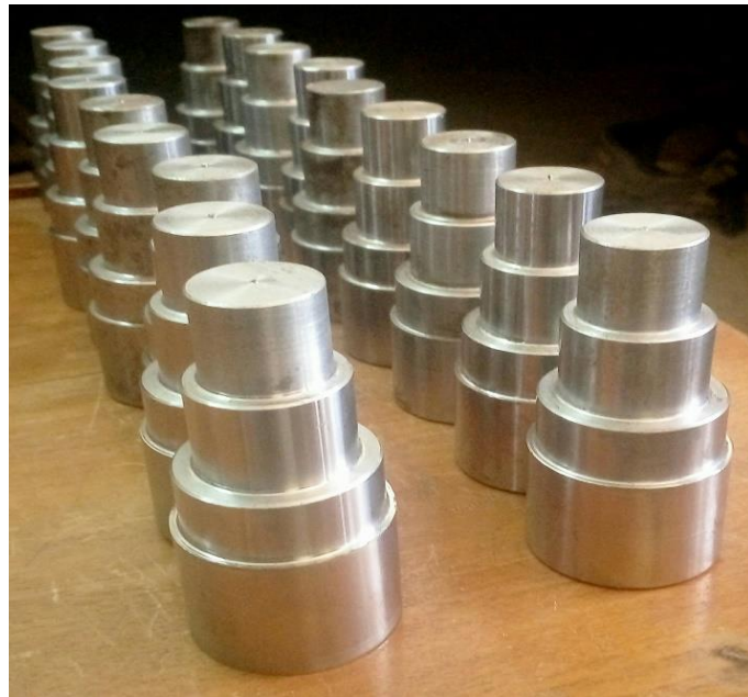
Fig2: CNC machined EN8 components.
